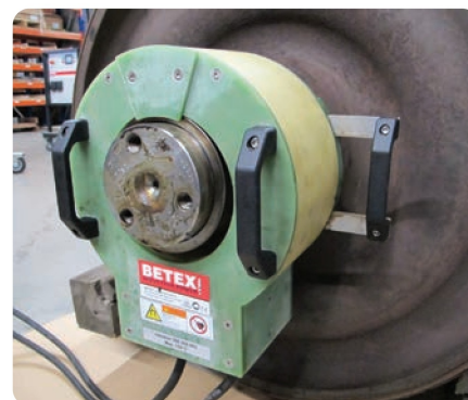
Heating bearing rings for dismantling
