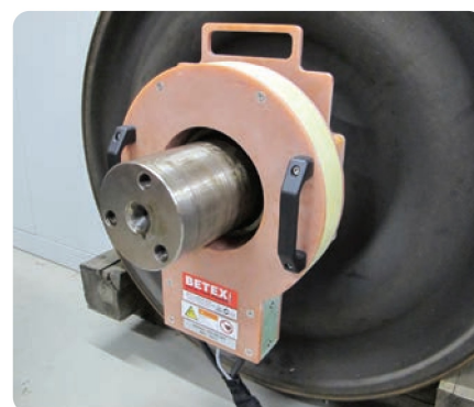
Heating labyrinth rings for dismantling
